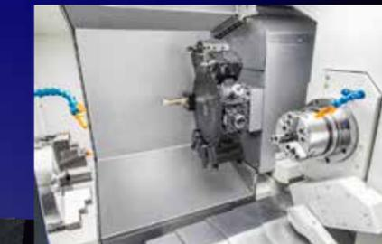
Main and Sub Spindle with Sauter BMT 65 Turret.
