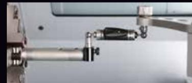
All XYZ PROTURN Lathes are thoroughly tested with the latest QC20 bluetooth Renishaw Ball Bar system.
