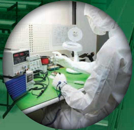
We provide IEC standards-compatible ESD protection items ranging from EPA working mats laid on workbenches, storage racks, and trolley surfaces, EPA flooring for PVC floors or floor coating, and to wrist straps for ESD countermeasures.
